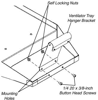
FIGURE 2 - INSTALLING THE VENTILATOR TRAY HANGER BRACKET ONTO THE VENTILATOR TRAY
